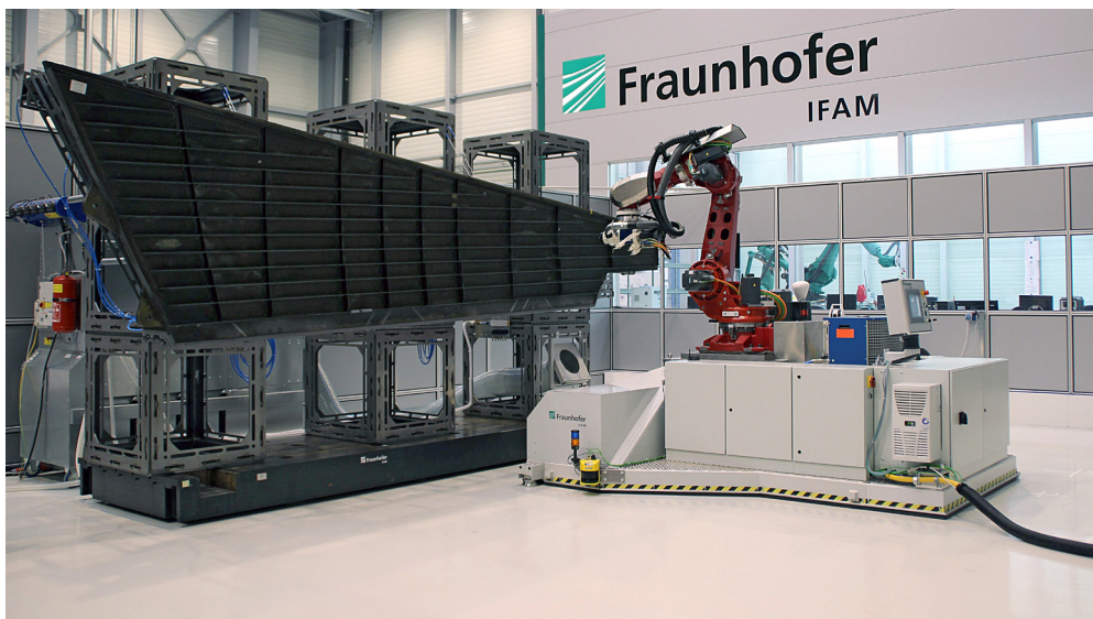
The mobile robot is processing the tail-fin of an Airbus 320 aircraft. © Fraunhofer IFAM | Picture in color and printing quality: www.fraunhofer.de/en/press
